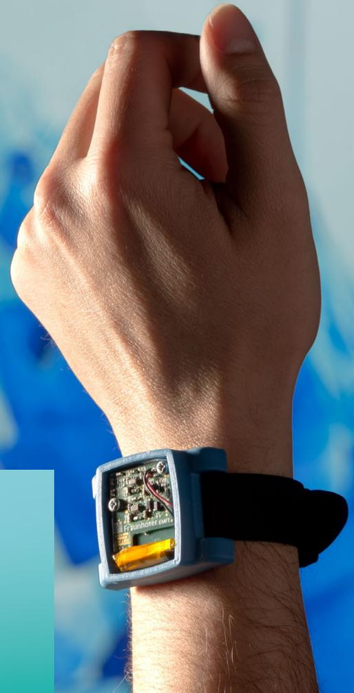
*Medical wearable: Sensor bracelet for vital parameter measurement and health detection*
