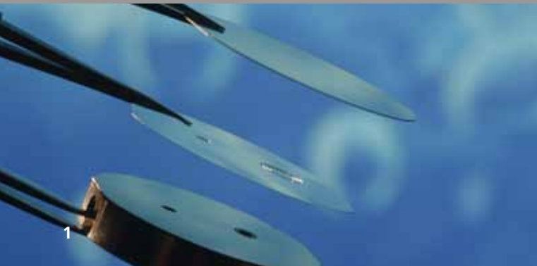
1 Multi layer joints of the stainless steel micropump
