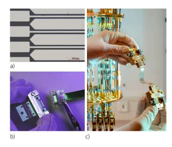
a) Conductor structures made of niobium on a polyimide substrate b) Superconducting interconnection of 10 signal lines via face-to-face transition
