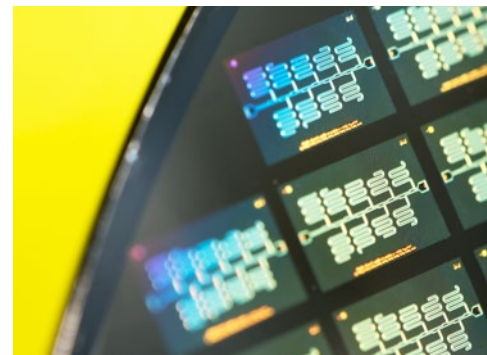
Resonators for material analysis for superconducting qubits on 200-mm wafers with Nb coating
