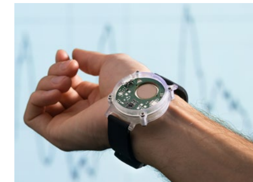
Portable blood pressure measurement using Fraunhofer EMFT micropumps
