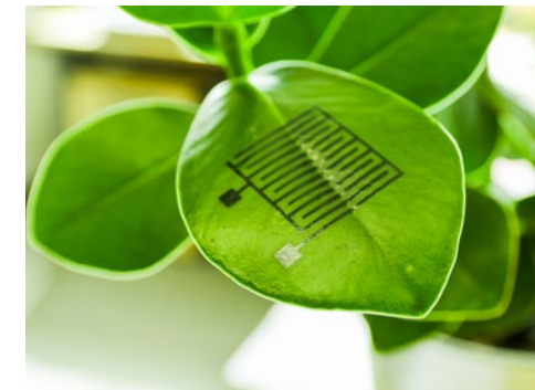
Sensors based on organic semiconductors for the monitoring of plant vitality and as indicators of parasitic infestation
