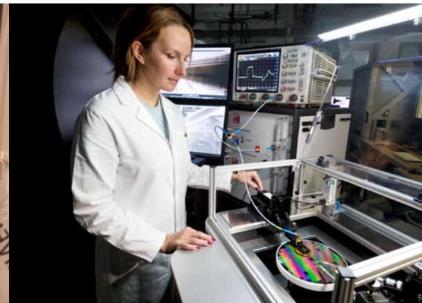
CC-TLP: original probe for capacitively coupled CDM-like TLP stress testing at wafer level
